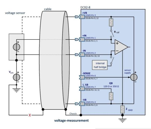
LEMO is the 7-pin LEMO DSUB 15-pin DSUB  $Z_{GND} \qquad \text{is ca. 500 k} \Omega \text{ for CRFX, else 0 } \Omega$
