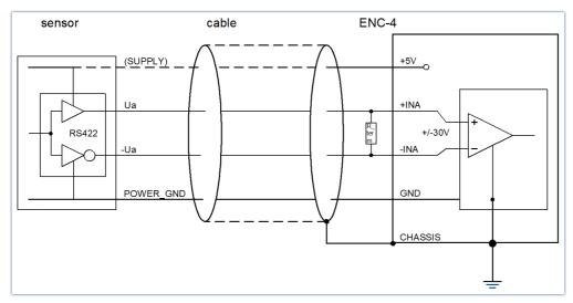
sensor with RS422 differential output
