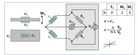
Longitudinal forces, torsion and temperature changes are compensated.
