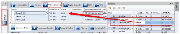
ICP expansion plug with TEDS information from the sensor or from the imc SENSORS database
