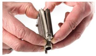
ACC/DSUBM-xxx: snap the nose into the slot
