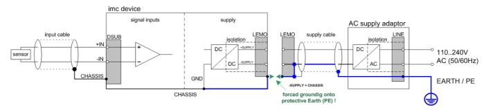
imc SPARTAN system with AC/DC power adapter
