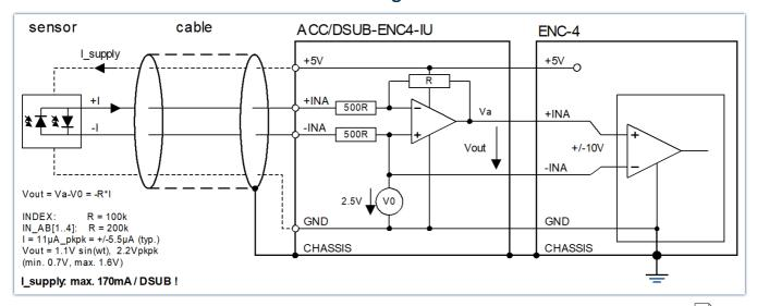
For a rotational encoder working with current signals, the current/voltage terminal ACC/DSUB-ENC-4-IU 182 can be used.
