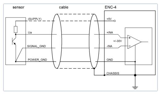
sensor with open-collector output
