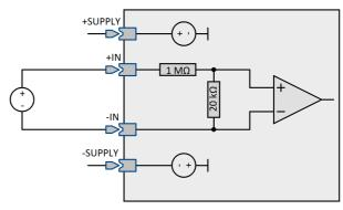
configuration for voltages >2 V with internal divider
