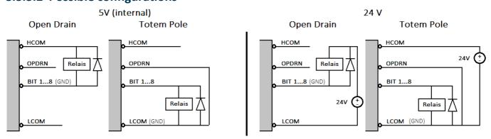
With **Totem Pole**, a maximum of **22 mA load current** is possible, totally independently of any externally connected voltage.
