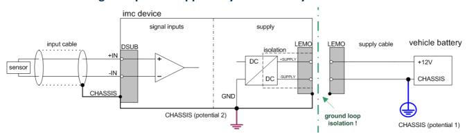
imc SPARTAN system with isolated from the housing (CHASSIS)) input with isolated DC-supply (e.g. battery)
