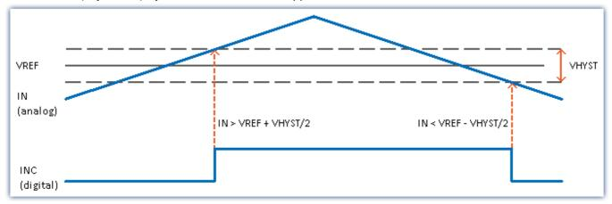
The digital signal changes from 0 to 1 when the analog signal exceeds the VREF + VHYST/2 threshold.
