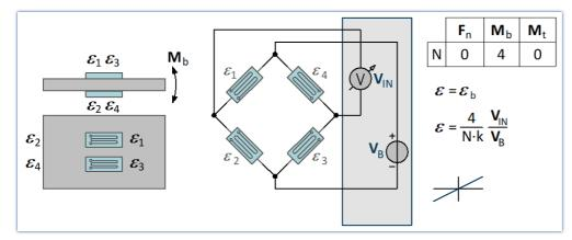
The sensitivity of the bending moment is increased. At the same time, longitudinal force, torque and temperature are compensated for.
