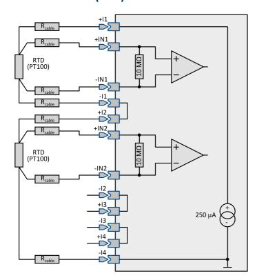
Along with Along with thermocouples, **PT100** sensors can also be connected, in **4-wire configuration**. An extra reference current source feeds an entire chain of up to four serially connected sensors.
