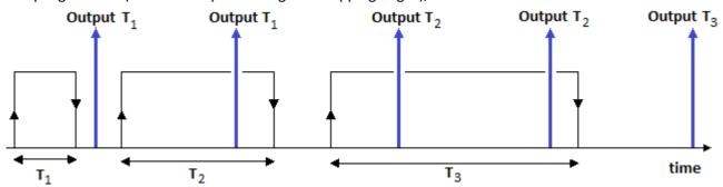
Above is illustrated a measured signal from which time readings are taken. Each reading starts at a positive edge in the signal and is stopped at a negative edge. The "up" arrows indicate the times at which the system returns a result. The returned values in this case are T1 –twice; T2 –twice; and T3.
