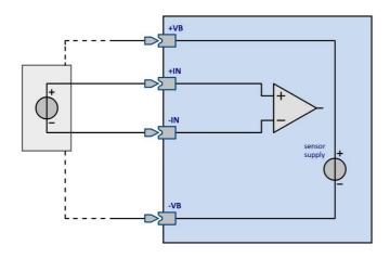
The sensor supply is unipolar and can be led out with DSUB-15 plugs at +VB and -VB (or +SUPPLY and -SUPPLY, see typing label in your plug). Only five selectable settings are available per module. The configurations can be taken from the respective module data sheet. The voltage can be set globally for all channels of a module. All channels of a module form a channel group.
