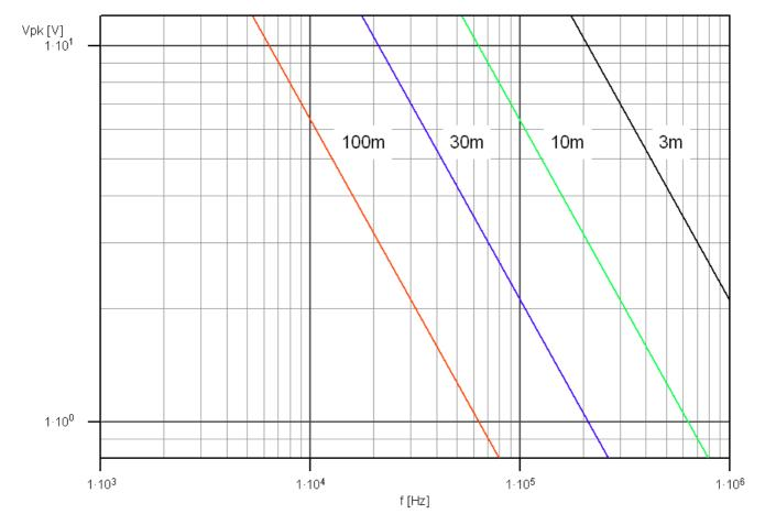
Maximum signal amplitudes as a function of the signal frequency and the cable length, with a 4 mA feed and a capacitance of 100 pF/m.
