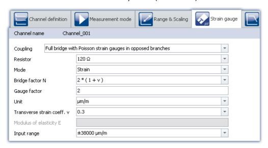
By selecting the "Strain gauge" measurement mode, common bridge circuits and strain gauge arrangements are offered. The scaling can be set using the typical parameters for strain measurements such as K-factor or transverse strain coefficient.
