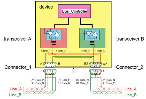
Internal wiring for EMD connection
