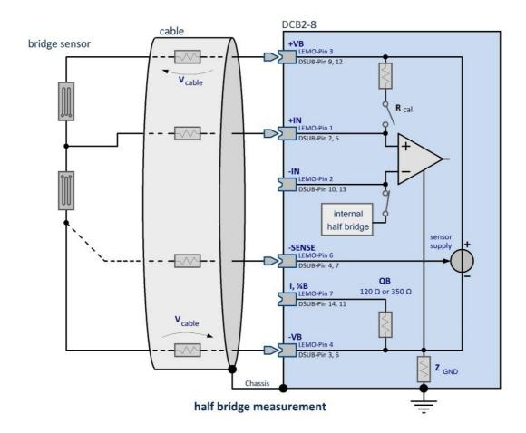
LEMO is the 7-pin LEMO DSUB 15-pin DSUB is ca. 500 k $\Omega$  for CRFX, else 0  $\Omega$
