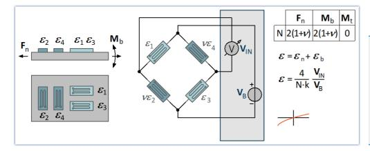
In this circuit, the specification of the transverse strain coefficient of the material is important. The arrangement is **insensitive** to temperature changes.
