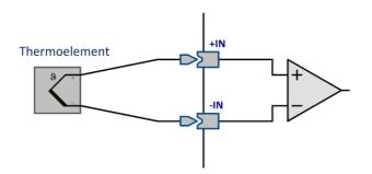
The common thermocouple types make use of linearization by characteristic curve.
