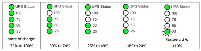
During active charging the last active one of the four green status LEDs flashes at a rate of approx one second. In contrast to this, the warning signal at very low state of charge (<10%) consists in the lowermost ("25") flashing at an even faster rate.
