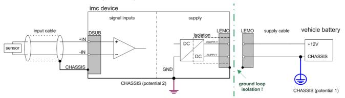
imc CRONOS-SL and imc CRONOScompact powered by an isolated DC-voltage source (e.g. battery)
