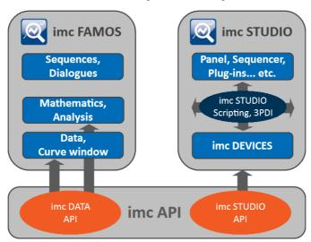
imc API offer a collection of .NET-components particularly designed to solve issues associated with measurement engineering and measurement data processing. The functionality provided covers broad ranges of the fields of managing, presenting and evaluating data. The components can be used by any Windows programming environment that supports .NET technology (C#, Managed C++, Visual Basic).
